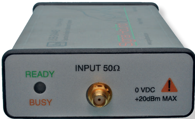
Front (above) and rear (right) panels of the Signal Hound USB-SA44B, just a bit larger than life size. There are no controls as such – they’re all taken care of via the supplied software.
