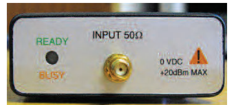
PHOTO 2: Front of SA44B analyser. The front of the TG44 tracking generator is similar.
