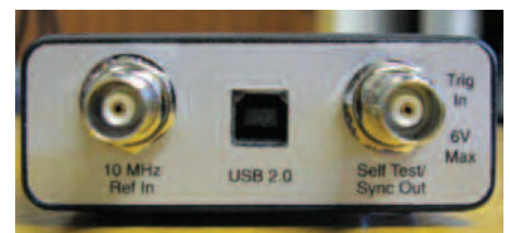
PHOTO 3: SA44B rear panel. The TG44 is similar.
