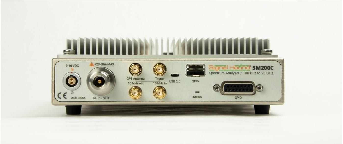
The SM200C is a high-performance spectrum analyzer and monitoring receiver with a 10 Gigabit Ethernet SFP+ port, which enables the SM200C to communicate with a PC over long distances using a fiber optic cable. Tuning from 100 kHz to 20GHz, the analyzer has 160 MHz of instantaneous streaming bandwidth (IBW), 110 dB of dynamic range, 1THz/sec sweep speed at 30kHz RBW (using Nuttall windowing), and phase noise performance that rivals even the most expensive spectrum analyzers on the market.
