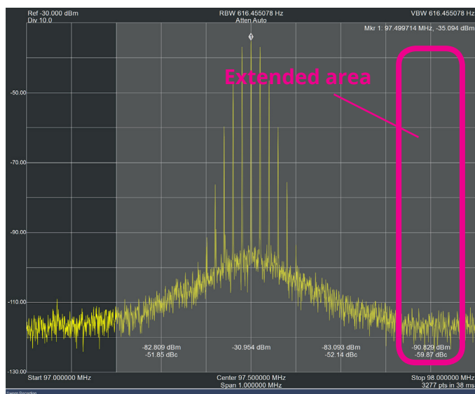
Figure 13—Changing the “Count” field in Spike Software to 4 or more extends the adjacent channel power ratio measurement beyond the immediately adjacent channels.
