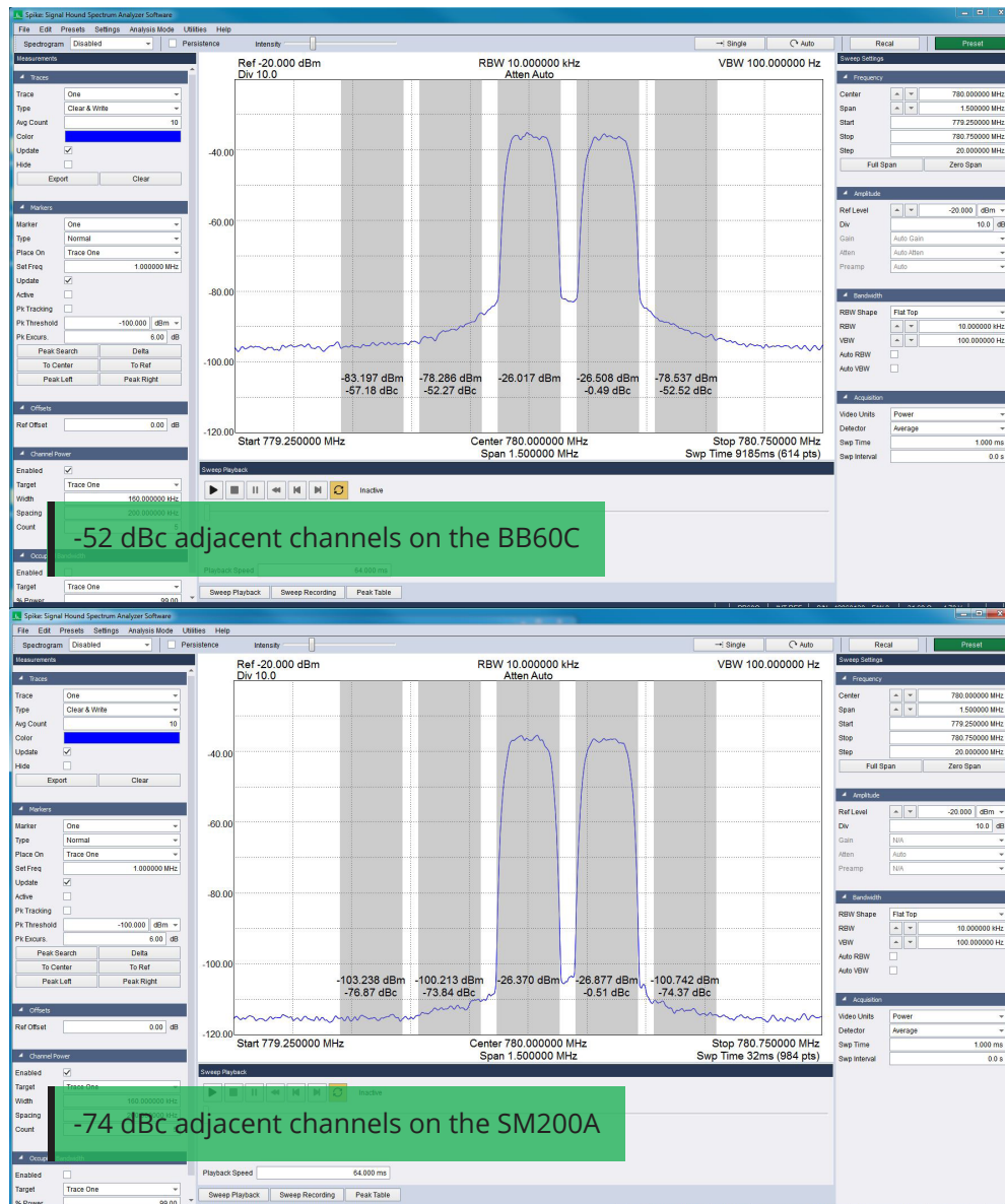
Figure 7—Adjacent Channel Power Ratio (ACPR) measurements. ( Note —Figure 7 shows the same signal being measured by both the BB60C and the SM200A. Note the 22dB lower noise floor achieved by the SM200A as compared to the BB60C. If you need the extra dynamic range for some of the more demanding ACPR measurements, then the SM200A will provide that needed performance.)
